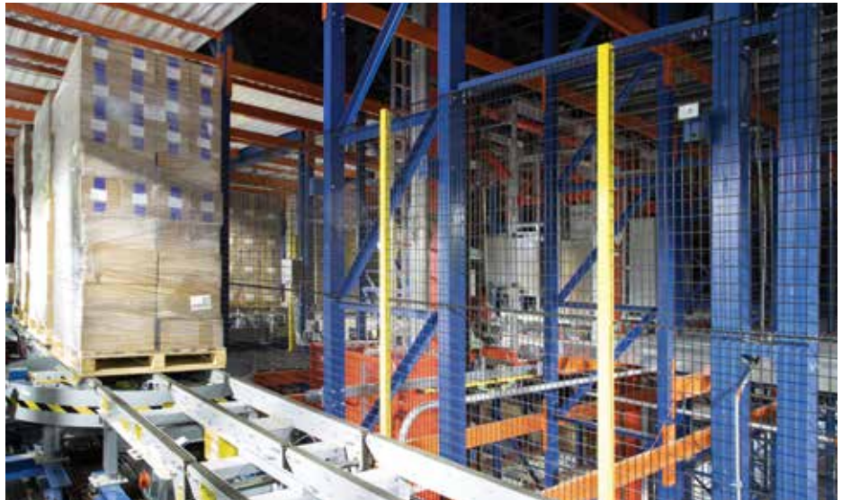
From truck to freezer, automated conveyors carry product throughout the conveyor tracks. (Photo courtesy of Fisher Construction Group.)
