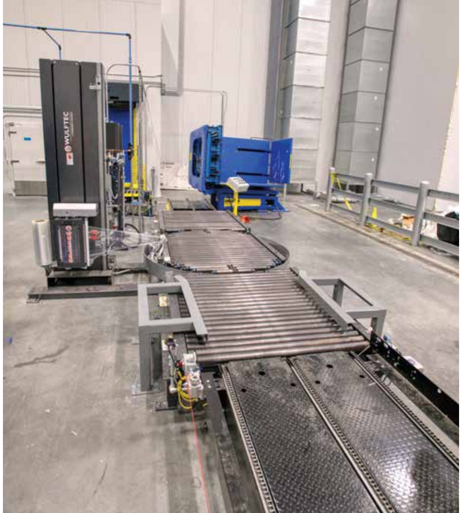
The facility features automated conveyors, wrapping and labeling stations. (Photo courtesy of Primus Builders.)
