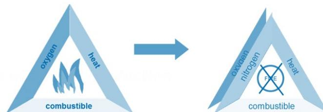
To what degree the oxygen needs to be lowered to prevent fire depends on the other two legs of the “three legged” stool. The temperature the controlled environment will be maintained at and the combustibility and other characteristics of the products occupying the space must be considered. Since it is proactive in nature and not required to penetrate and extinguish a raging fire that has somehow broken out, the methods and heights for storing materials becomes irrelevant.
