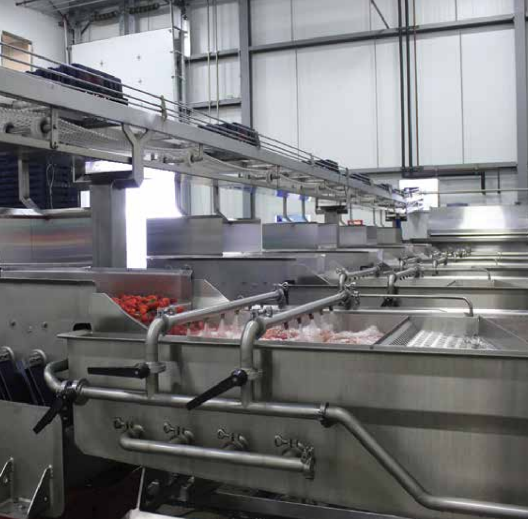
Left: Berries are cleaned and sorted before entering the clean processing room through wall opening. (Photo courtesy of Fisher Construction Group.)
