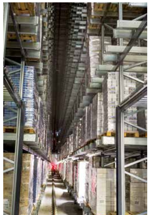
Left: The second fully automated high bay cold facility in the States is under construction in Idaho. Right: The facilities rely on automated storage and retrieval systems to move and store product in the high-bay warehouse. (Photos courtesy of NewCold.)
