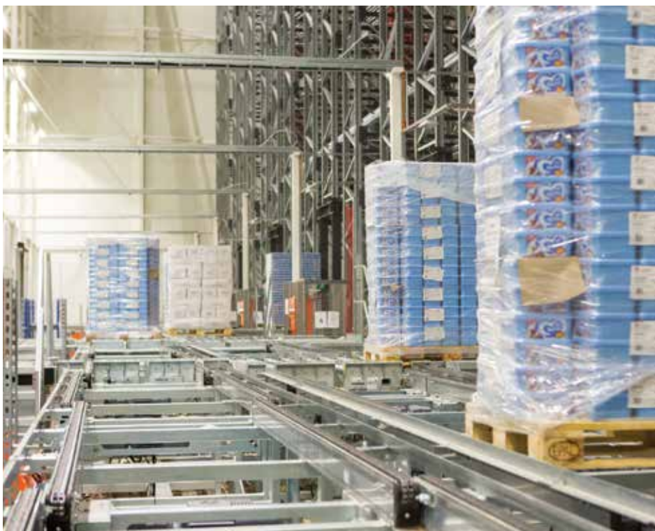
The ability to reduce use of conveyors in fully automated facilities leads to energy efficiencies. (Photo courtesy of NewCold.)
