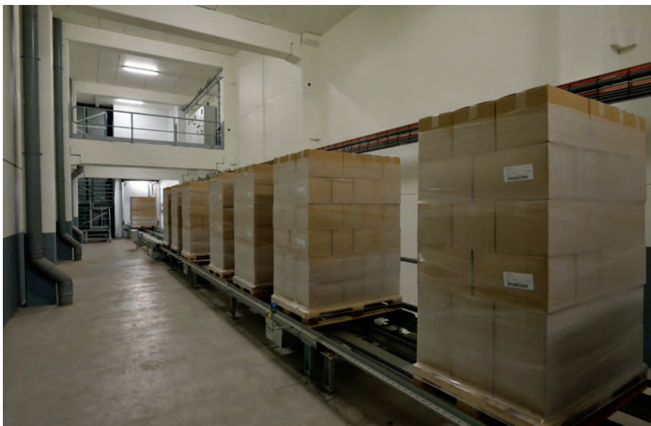
Agristo estimated a five-year return on investment for the automated warehouse, which uses conveyor systems to move product from production areas to refrigerated storage. (Photo courtesy of Egemin Automation.)
