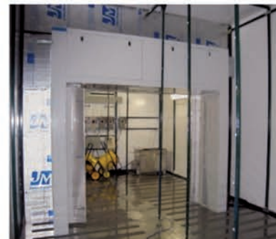
The HCR calorimetric environmental test chamber at CTS Labs in Urbana, IL
