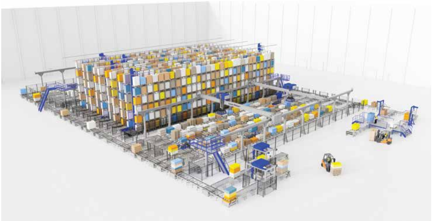
Left: High-density pallet shuttle ASRS facility that uses fixed-position vertical lifts and aisle carriers and row carriers on each level for high volume/high velocity facility with high throughput capabilities. (Photo courtesy of Primus Builders, Inc.)
