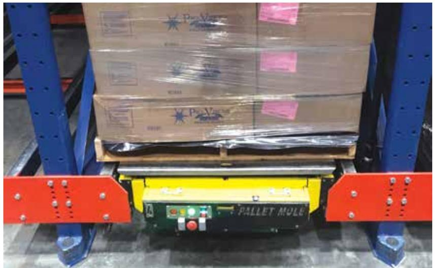
*The Pallet Mole® was utilized for over 150,000 cubic feet of space comprised of 76 bays of rack with 22 pallet deep aisles at the Nor-Am facility. (Photo courtesy of Frazier Industrial Company.)*
