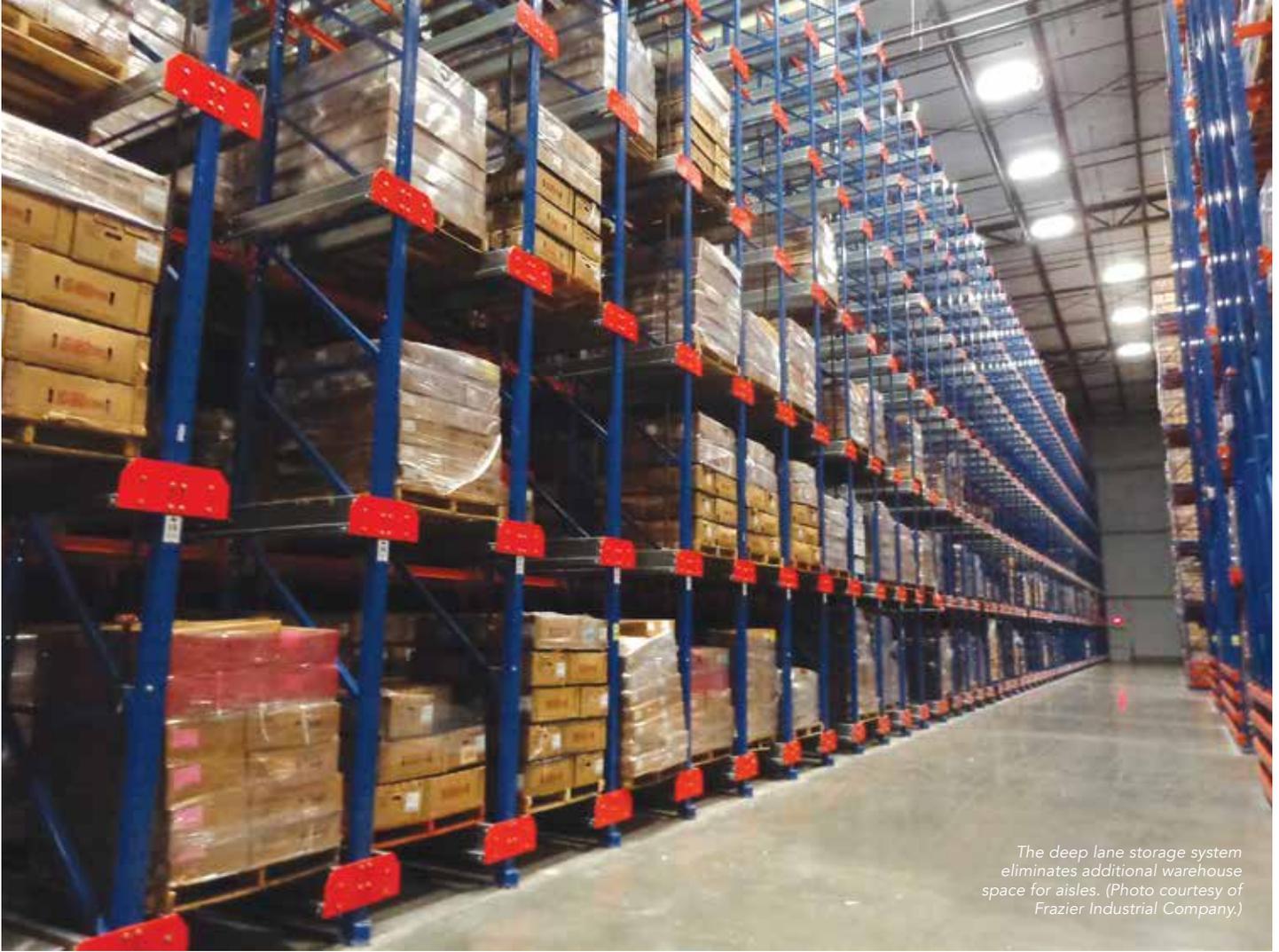
The deep lane storage system eliminates additional warehouse space for aisles. (Photo courtesy of Frazier Industrial Company.)
