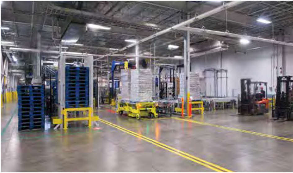
Automatic Guided Vehicles (AGVs) move, load, and unload pallets by themselves, like robots. (Photo courtesy of Primus Builders.)
