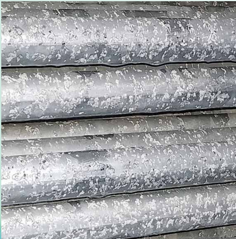
White Rusted Coil without Pass-Protect
