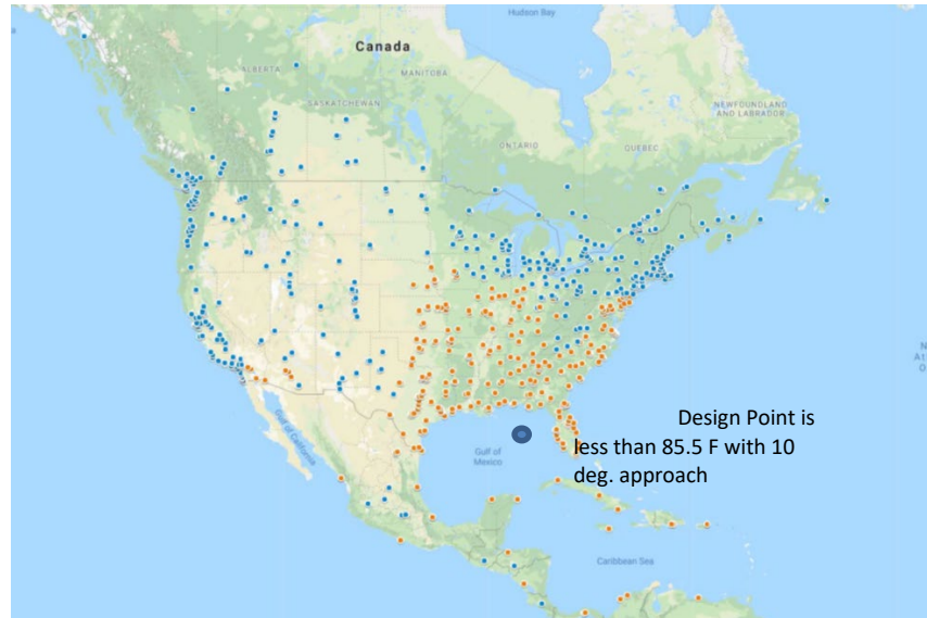
Figure 12: Regions of North America With No Hours in a Year of Supercritical Operation When Using Adiabatic Coolers ( )
