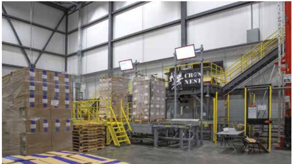
The conveyers are operated from a crow nest that can regulate product flow between the loading dock and freezers. (Photo courtesy of Fisher Construction Group.)
