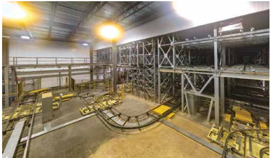
The subsystems were connected by an Electrified Floor Track System by Eisenmann, which moves product between locations and then to the shipping dock. (Photo courtesy of Griffco Design/Build.)
