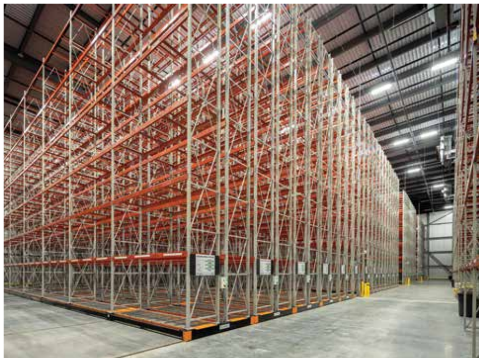
Flex space mobile racking in the finished facility. (Photo courtesy of Ti Cold.)
