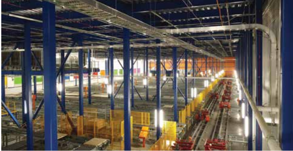
Once a pallet is unloaded, it is placed on an inbound conveyor where the system tracks each pallet and designates it a position in the freezer. (Photo courtesy of Fisher Construction Group.)
